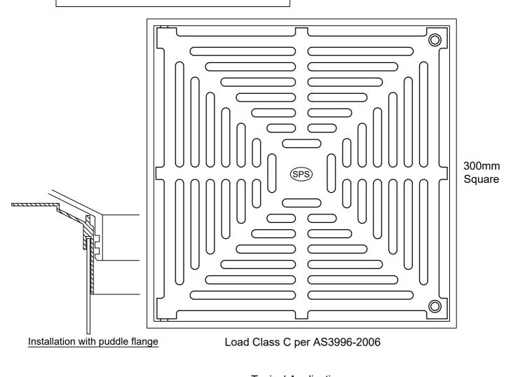
Typical Applications Tiling or topping ₩2 Z Ľ  $\square$ Δ 0 Min. height 45mm 80mm Structural Slab <1200mm  $\triangleleft$ I.D. rubber ring seals Strainer Basket Standard PVC Pipe Code: SBV85 to suit 100mm PVC, 2mm holes HDPE & copper  $\triangleleft$ With topping/tiling Cast into slab
